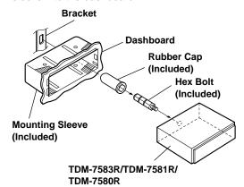
When your vehicle has the Bracket, mount the long hex bolt onto the rear panel of the TDM-7583R/TDM-7581R/TDM-7580R and put the Rubber Cap on the hex bolt. If your vehicle does not have the Mounting Support, reinforce the head unit with the metal mounting strap (not supplied). Connect all the leads of the TDM-7583R/TDM-7581R/TDM-7580R according to details described in the CONNECTIONS section.
